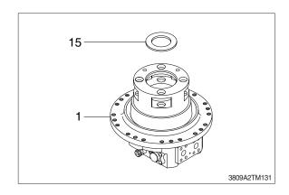
(3) Insert the assembly of hub (3) to track motor (1).
