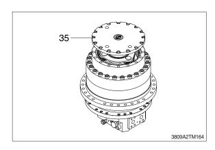
(25) Assemble cover (35) and tighten them to the specified torque.
