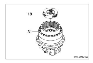
(18) Assemble plate (36) to carrier B (18).
