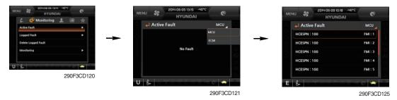
· The active faults of the MCU, engine ECM, air conditioner or AAVM can be checked by this menu.
