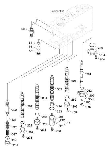
155 Plug 273 Hex screw 394 Am/Confluence spool kit 165 O-ring 301 Travel spool kit 551 Plug 202 Spring cover 303 Boom spool kit 561 O-ring 208 Spool cover 304 Bucket spool kit 603 Port relief assy 211 Plug 313 Plug 611 Negative relief valve assy 212 O-ring 326 Spring 754 Flange 251 Plug 327 Spring O-ring 763 262 O-ring 337 Rod 764 Socket screw 263 O-ring 391 Travel straight spool kit 265 O-ring 392 By pass cut spool
