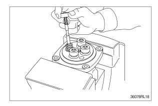
(3) Assemble O-ring (10) onto plug (8).
