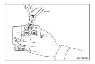
(11) Fit set spring (655) to spool hole and put compensating piston (621) and piston case (622) into compensating hole.
