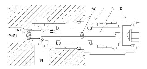
③ The oil flow chamber g via orifice m and n. When the pressure chamber g reaches the preset force (Fsp) of spring (4), the piston (6) moves left and stop the piston (6) hits the bottom of sleeve (7).
