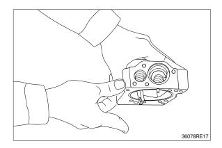
(13) Install cover (C, 629) fitted with adjusting screws (628), adjusting stem (C, 627), lock nut (630), hexagon nut (802) and set screw (924).
