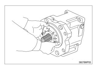
(11) Tapping lightly fitting flange section of swash plate support (251) on its pump casing side, separate swash plate support from pump casing.
