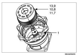
(12) Assemble the three friction plates (14) and four separation plates into the casing (1).
