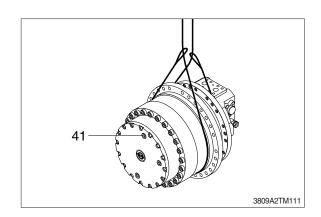
(2) After loosening drain plug (41), drain gear oil.
