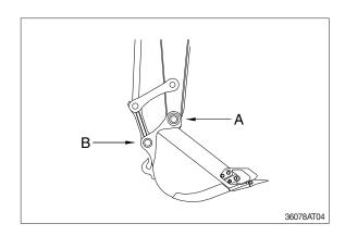
② Remove nuts (1), bolt (2) and draw out the pin (B).
