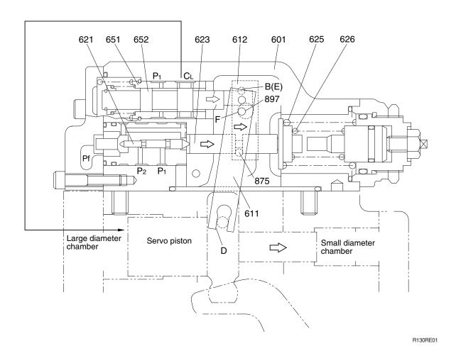
When the self pump delivery pressure P1 or the companion pump delivery pressure P2 rises, it acts on the stepped part of the compensating piston (621). It presses the compensating rod (623) to the right till the force of the outer spring (625) and inner spring (626) balances with the hydraulic force. The movement of the compensating rod is transmitted to lever 1 via pin (875). Lever 1 rotates around the pin (875) (E) fixed to the casing (601).
