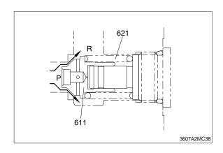
The relation between the flow rate Q and pressure P of the hydraulic oil that flows from the path (P) to the low-pressure path (R) is as shown in the diagram.
