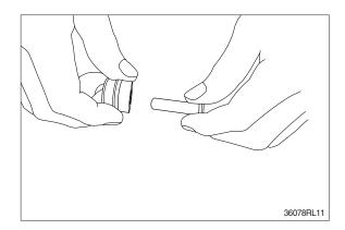
(13) Remove O-ring (10) and seal (11) from plug (8).
