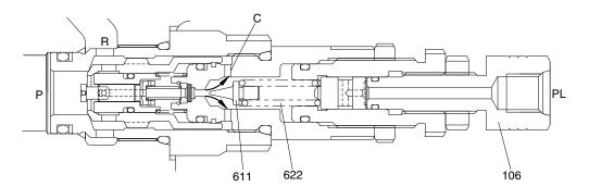
③ Opening of the poppet (611) causes the pressure in chamber B to fall and the plunger (511) to open. As the result the pressurized oil in the path (P) runs into the low pressure path (R) directly.
