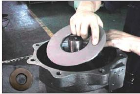
6 Using a plier jig, disassemble snap ring (4) and shaft assy (5).
