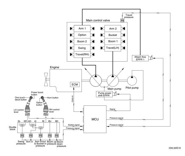
1. When the requirement of pump flow rate is low, IPC mode controls pump flow rate to improve fuel efficiency.
