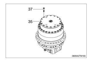
(26)Inject gear oil and assemble plug (41) of cover (35).
