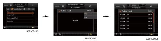
$\cdot\,$  The active faults of the MCU or engine ECM can be checked by this menu.
