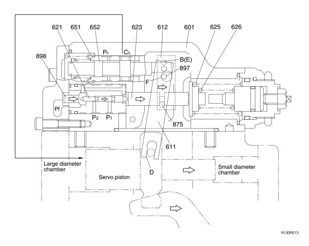
The set horsepower valve is shifted by varying the command current level of the proportional pressure reducing valve attached to the pump.
