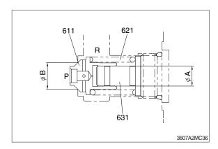
② In this condition, the pressurized oil in the path (P) runs out to the path (R) through the orifice (c).
