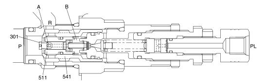
② When the pressure in the path (P) becomes equal to the set pressure of the spring (621 or 622), the pressurized oil pushes open the poppet (611), flows around it, and flows to the low pressure path (R) through Hole C.
