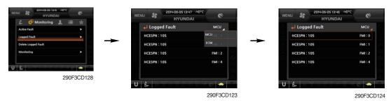
• The logged faults of the MCU, engine ECM, air conditioner or AAVM can be checked by this menu.
