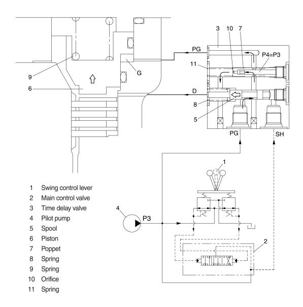
b. When all of the RCV lever (1) are set the neutral position, the spool (5) returns to right. Then, the piston (6) is moved lower by spring force and the return oil from the chamber G flows back to tank port.
