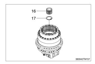
(17) Assemble carrier B (18) to ring gear (31).
