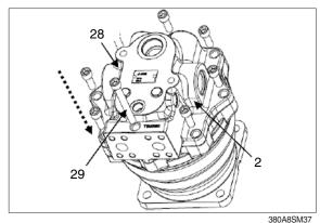
(20) Assemble the spring (20) and RO plug (21) into the valve casing (2) after seat making the plunger (19) on the valve casing (2) two or three times.
