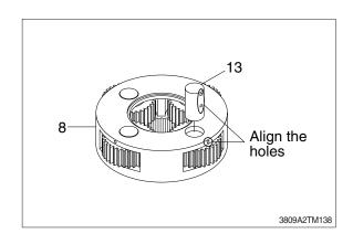
Assemble carrier (8) and pin (13) striking pin (14) by hammer.After assembly pin (14), caulking.
