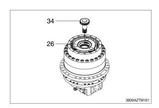
(22) Assemble plate (36) to carrier C (26).
