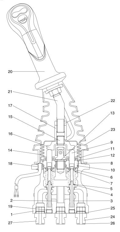
Plug Case Joint assembly 22 Nut 1 8 15 2 **Bushing** 9 Push rod 16 Swash plate 23 Boot Adjusting nut Last guard filter 3 Spool 10 O-ring 17 24 Bushing 4 Shim 11 Rod seal 18 25 O-ring Plate 5 Spring 12 19 Plug 26 O-ring 6 Spring seat Spacer Handle assembly 27 Connector 13 20 7 Boot 21 Handle bar Spring 14
